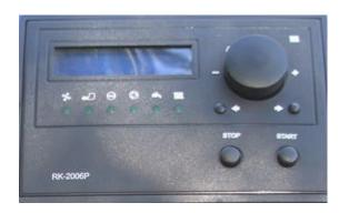
. The main window, the mode of regulation and the status of output devices. After power controller displays the main window. The top line of the display () is shown in the boiler water temperature, in the lower, work mode. (\*); Symbol appears in the lower right corner of the detection of flame in the burner. Lights below the display are assigned to the corresponding outputs, and steady light indicates the status of their activation.
